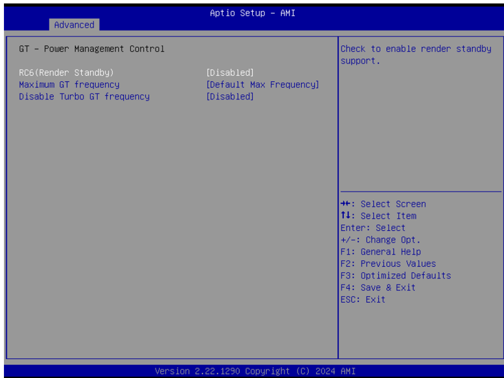
Figure 5.8 GT- Power Management Control
