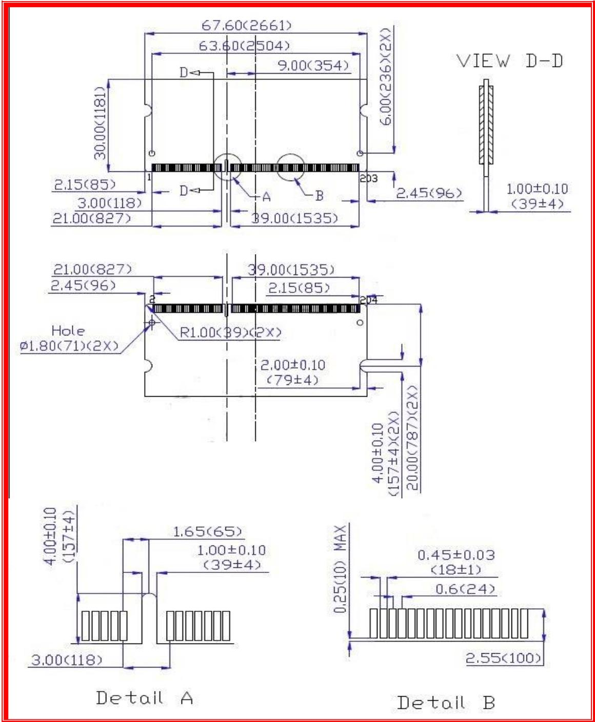
Note: All dimensions are in millimeters (mils) and should be kept within a tolerance of ±0.15 (6), unless otherwise specified.
