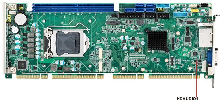
This HDAUD1 pin header is the connection interface to Advantech's high definition audio module.
