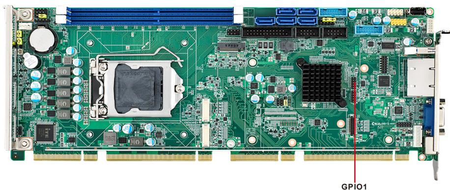
Provides 10-pin header connector for 8-bit Digital I/O usage. Refer to Appendix B for detailed information on the pin assignments and programming guide in Appendix C.
