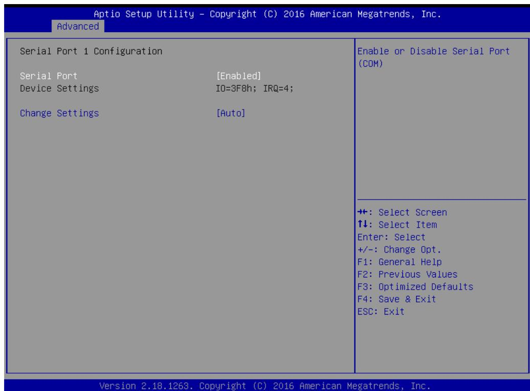
Figure 3.17 Serial Port 1 Configuration
