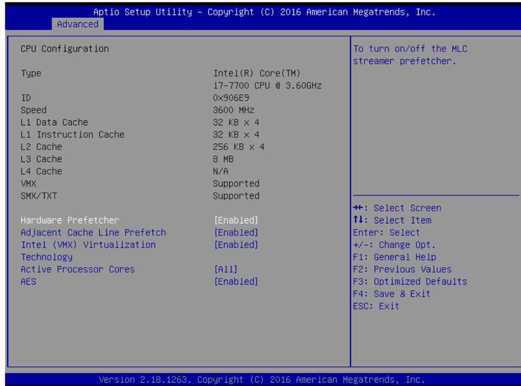
Figure 3.5 CPU Configuration
