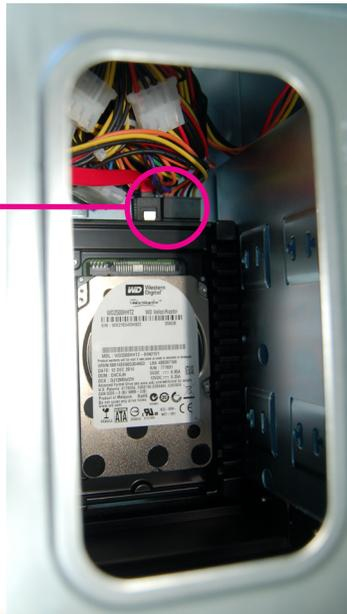
4. Secure the HDD bracket back to the system.
