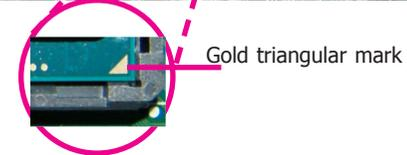
**Important:** The CPU will fit in only one orientation and can easily be inserted without exerting any force.
