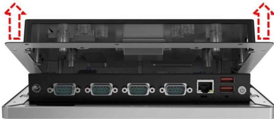
Figure 3-2: Remove the Back Cover
