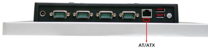
Figure 3-6: AT/ATX Switch Location
