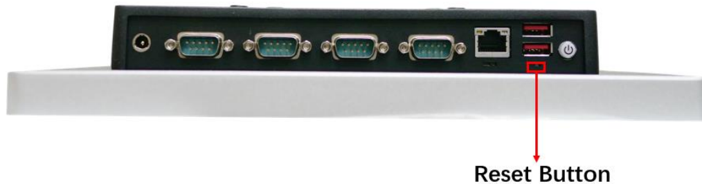
Figure 3-17: Reset Button Location
