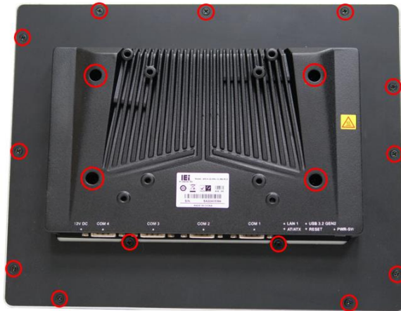
Figure 3-1: Back Cover Retention Screws
