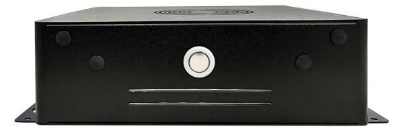
The above shows the power button at the center and four antenna screw holes.
