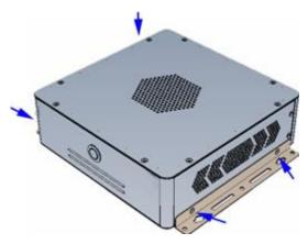
2. Then prepare at least four screws (M3, 6 mm) to mount the device on the wall.
