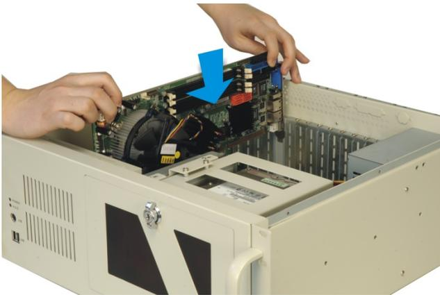
**Figure 9: Slide the CPU Card into the Sockets**
