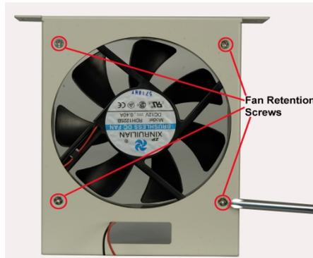
**Figure 18: Remove the Fan Retention Screws**
