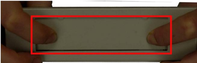
**Figure 16: Bend off the front cover of the 3.5" drive bracket**
