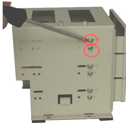
**Figure 13: Remove the 3.5" Drive Tray Retention Screws**
