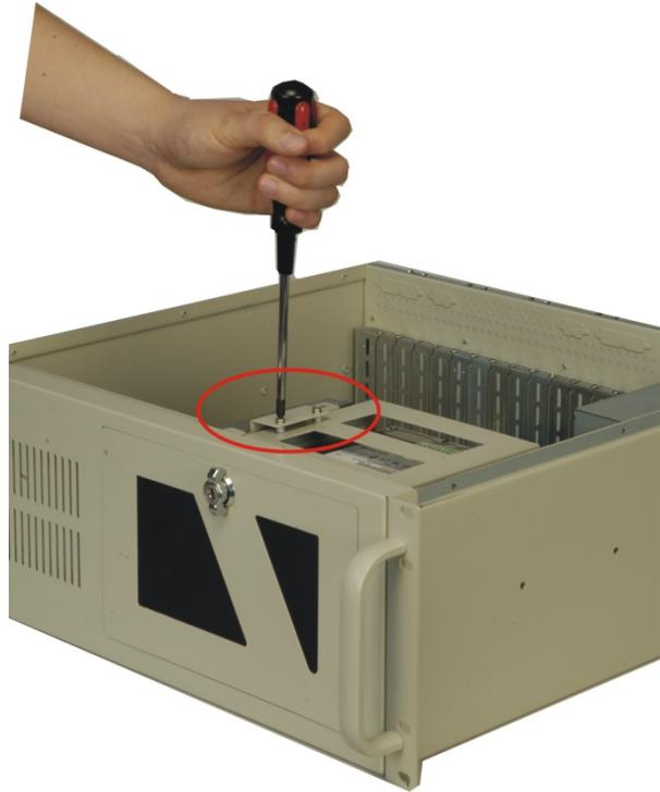
**Figure 10 Remove the Side Bracket**
