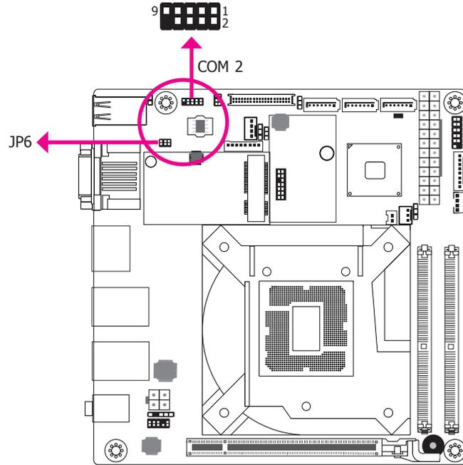
JP6 is used to configure COM 2 to pure RS232 or RS232 with power. The pin functions of COM 2 will vary according to JP6's setting.
