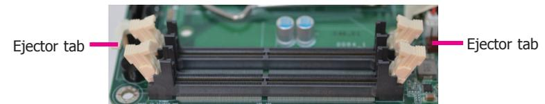
5. Note how the module is keyed to the socket.
