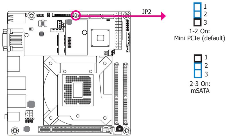
JP2 is used to select the Mini PCIe signal.
