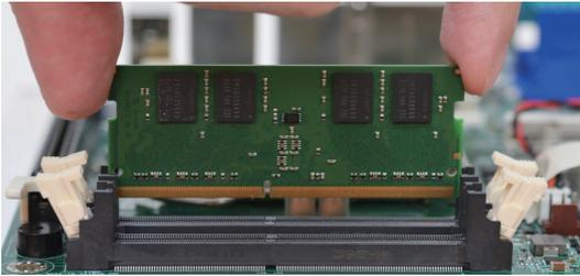
7. Seat the module vertically, pressing it down firmly until it is completely seated in the socket. The ejector tabs at the ends of the socket will automatically snap into the locked position to hold the module in place.
