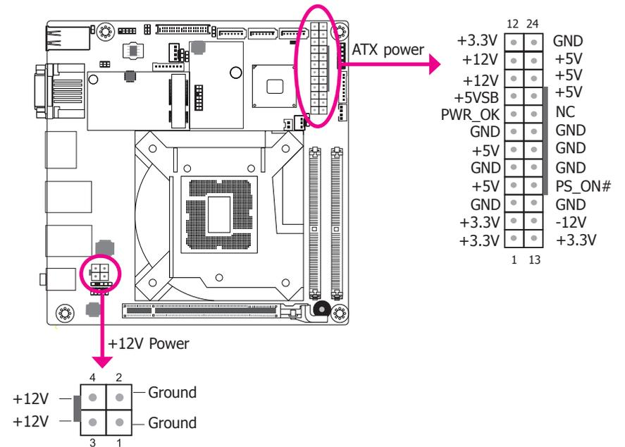
Use a power supply that complies with the ATX12V Power Supply Design Guide Version 1.1. An ATX12V power supply unit has a standard 24-pin ATX main power connector that must be inserted into the 24-pin connector. The 4-pin +12V power connector enables the delivery of more +12VDC current to the processor's Voltage Regulator Module (VRM).
