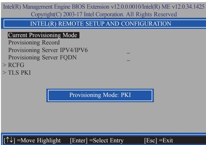
41. In the **Intel(R) Remote Setup And Configuration** menu, select **Provisioning Server IPV4/IPV6** then press Enter. Enter the address then press Enter.
