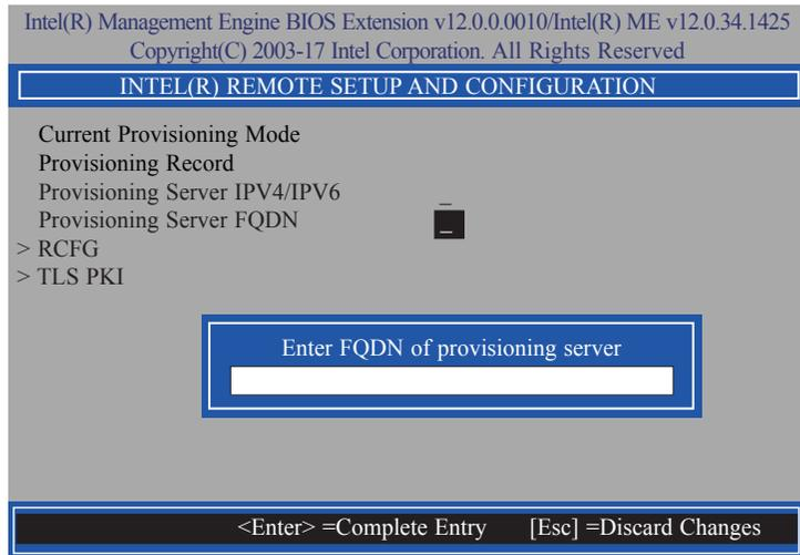
43. If you want to activate remote configuration, in the **Intel(R) Remote Setup And Configuration** menu, select **RCFG** then press Enter. Select **Start Configuration** then press Enter. Press Y to activate.
