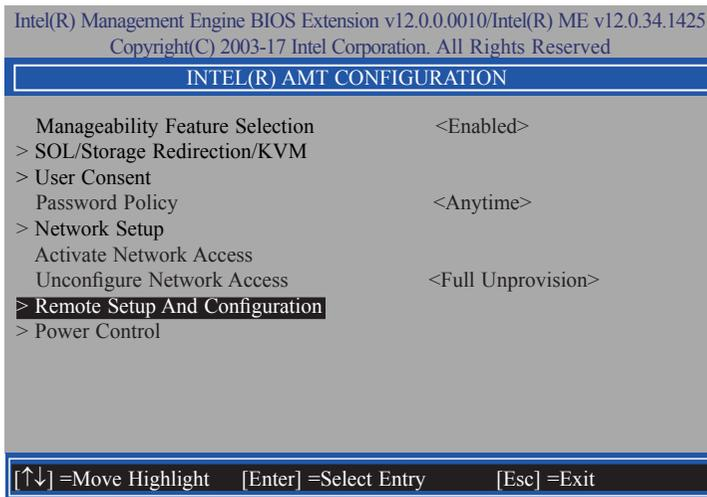
40. In the **Intel(R) Remote Setup And Configuration** menu, select **Provisioning Record** then press Enter.
