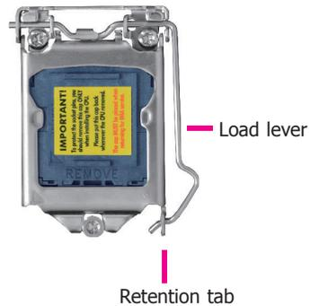
5. Lifting the load lever will at the same time lift the load plate.
