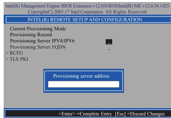
42. In the **Intel(R) Remote Setup And Configuration** menu, select **Provisioning Server FQDN** then press Enter. Enter the FQDN then press Enter.
