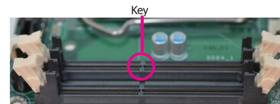
6. Grasping the module by its edges, position the module above the socket with the “notch” in the module aligned with the “key” on the socket. The keying mechanism ensures the module can be plugged into the socket in only one way.
