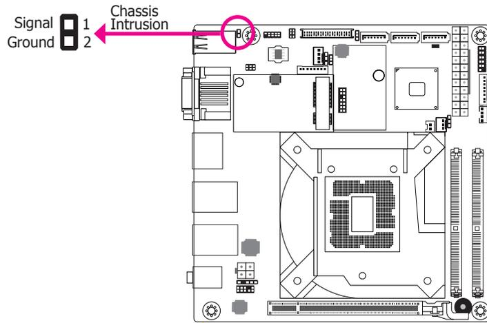
The board supports the chassis intrusion detection function. Connect the chassis intrusion sensor cable from the chassis to this connector. When the system's power is on and a chassis intrusion occurred, an alarm will sound. When the system's power is off and a chassis intrusion occurred, the alarm will sound only when the system restarts.
