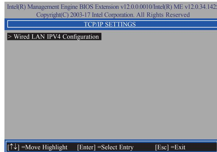
30. In the **Wired LAN IPv4 Configuration** menu, select **DHCP Mode** then press Enter. Select **Enabled** or **Disabled** then press Enter. If set to **Disabled**, **IPV4 Address**, **Subnet Mask Address**, **Default Gateway Address**, **Preferred DNS Address** and **Alternate DNS Address** will show up.
