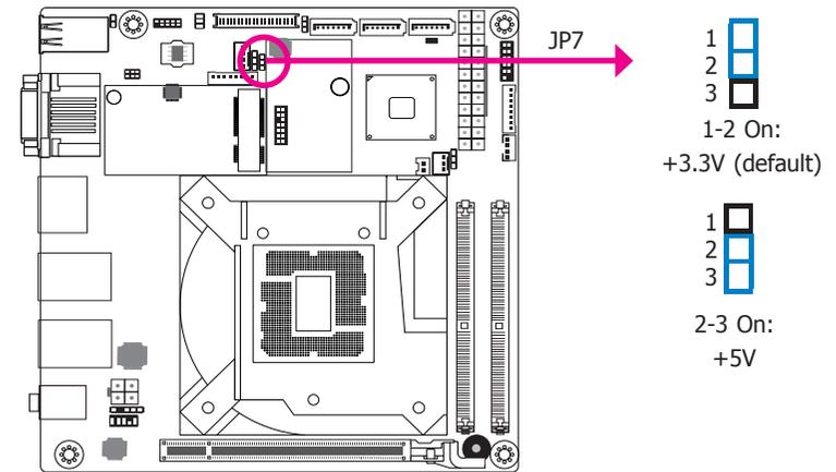
JP7 is used to select the power level of backlight brightness control: +3.3V (default) or +5V.
