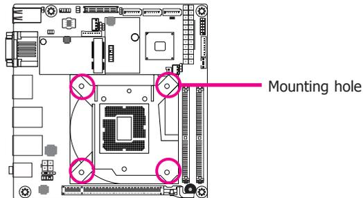
3. Orient the heat sink such that the CPU fan's cable is nearest the CPU fan connector.
