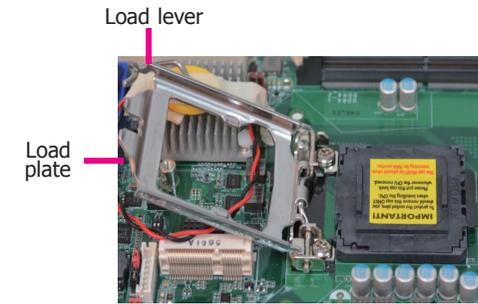
6. Remove the protective cap from the CPU socket. The cap is used to protect the CPU socket against dust and harmful particles. Remove the protective cap only when you are about to install the CPU.
