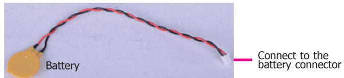
The lithium ion battery powers the real-time clock and CMOS memory. It is an auxiliary source of power when the main power is shut off.
