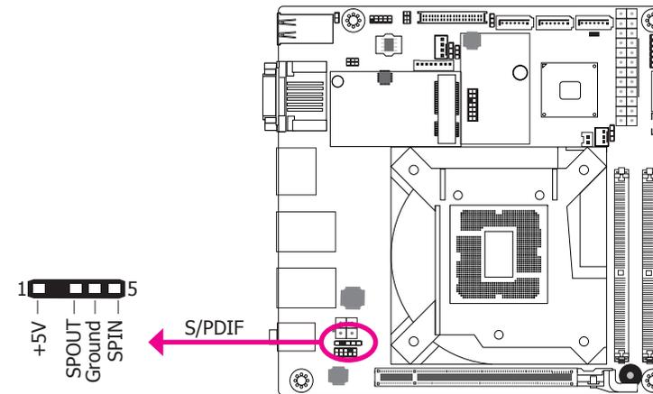
The S/PDIF connector is used to connect an external S/PDIF port. Your S/PDIF port may be mounted on a card-edge bracket. Install the card-edge bracket to an available slot at the rear of the system chassis then connect the audio cable to the S/PDIF connector. Make sure pin 1 of the audio cable is aligned with pin 1 of the S/PDIF connector.
