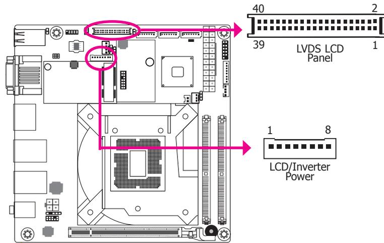
The system board allows you to connect a LCD Display Panel by means of the LVDS LCD panel connector and the LCD/Inverter power connector. These connectors transmit video signals and power from the system board to the LCD Display Panel.
