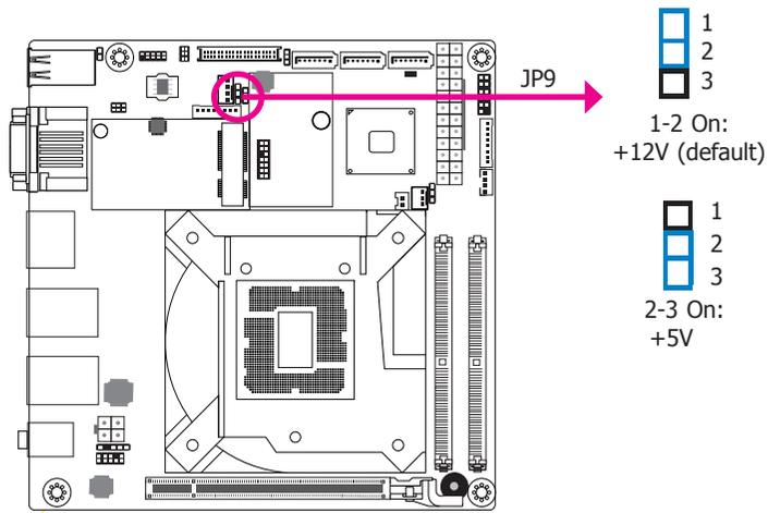
JP9 is used to select the power level of LVDS LCD inverter connector.
