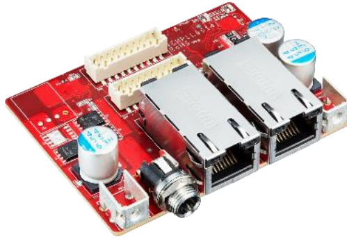
Figure 5: Mounting Hole, DC Jack, Daughter Board Picture (EGPL-G2P1-C7/W7)
