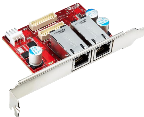
Figure 4: Bracket, 4Pin Header, Daughter Board Picture (EGPL-G2P1-C6/W6)
