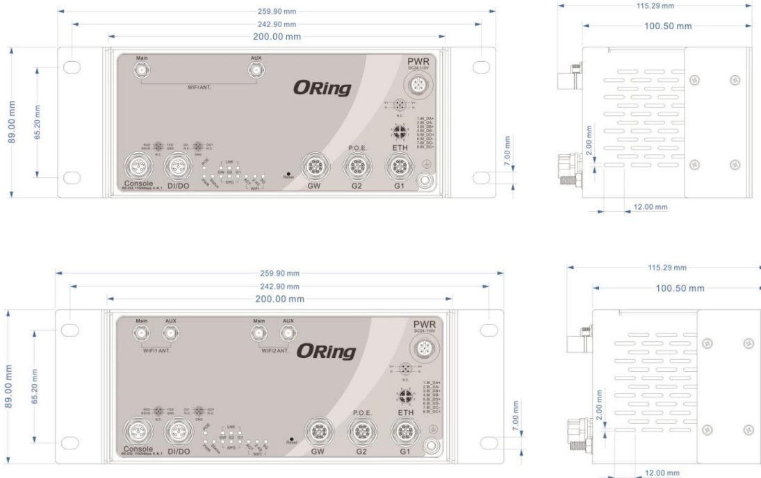
Rack-Mount Kit Measurement (Unit = mm)
