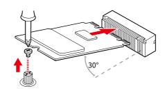
2. Secure the M.2 SSD in place with the supplied M.2 screw.
