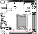
PCIE1: PCIe 5.0 x16 (signal from CPU)
