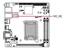
1. Insert your M.2 SSD into the M.2 slot at a 30-degree angle.
