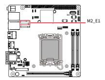
Please install the Wi-Fi/ Bluetooth card into the M.2 slot as shown below.
