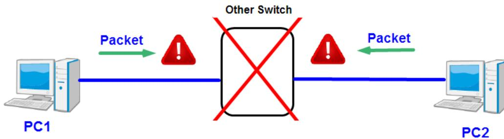
Switches with bypass functions such as the Bypass Switch provide one or more sets of bypass ports that ensure constant network connectivity during power failure.
