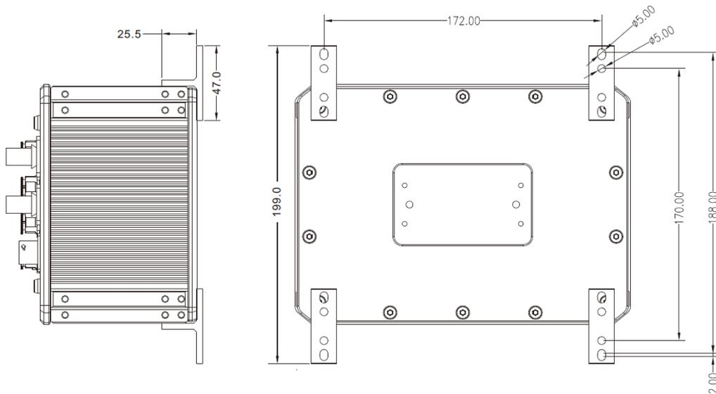
Wall-mount Measurement (Unit = mm)
