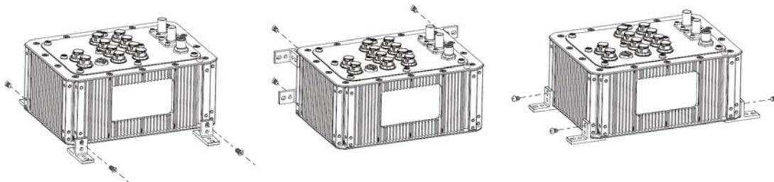
Step 2: Hold the device upright against the wall.
