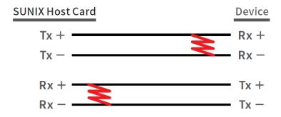
2-Wire RS-485 working model with termination resistor:
