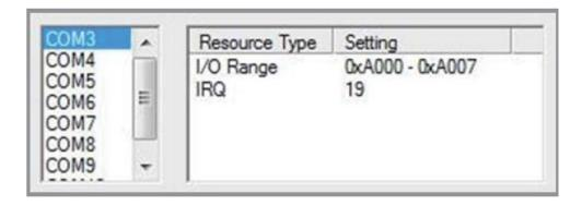
IRQ and I/O address is automatically assigned by the mainboard PCI (PCI Express) BIOS automatically (before COM card driver installing). User can NOT assign legacy ISA address (3F8, 3E8, 2F8, 2E8) for the specific COM port. But for IRQ setting, user can set specific IRQ value for this PCI Express bus slot via mainboard's BIOS settings (not via SUNIX driver). But all COM ports will share one IRQ value.
