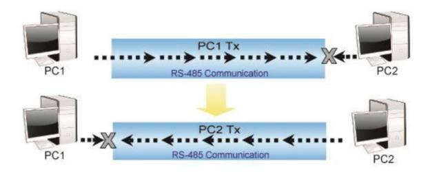
Auto Carrier Sense (ACS™) technology will check the status of RS-485 communication bus. If the bus is idle, it starts transmission. If the bus is not idle (some data flows in the bus), then it will postpone the transmission of UART until the bus is idle. Due to the reduction of TX/RX packet conflicting on RS-485 one-way traffic bus, it will enhance better system performance and RS-485 communication ability.
