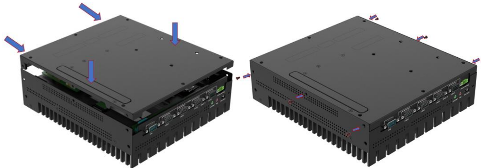
Figure 3-13: Back Cover Installation
