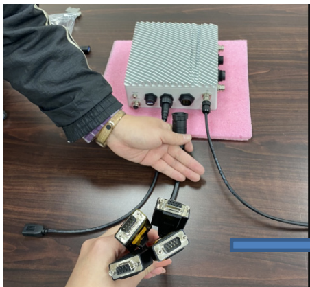
23pin 1to4 converter cable to connect ECX700 and cables of RS232 or CAN devices
