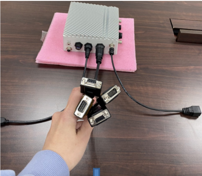
This is a standard 23pin 1to4 converter cable after assembly; customer can either use our converter cable or a customized cable to directly connect ECX700 with their devices
