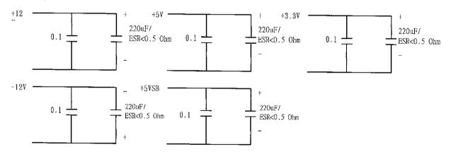
0.1uf is ceramic the other is tantalum. Noise bandwidth is from DC to 20MHz
