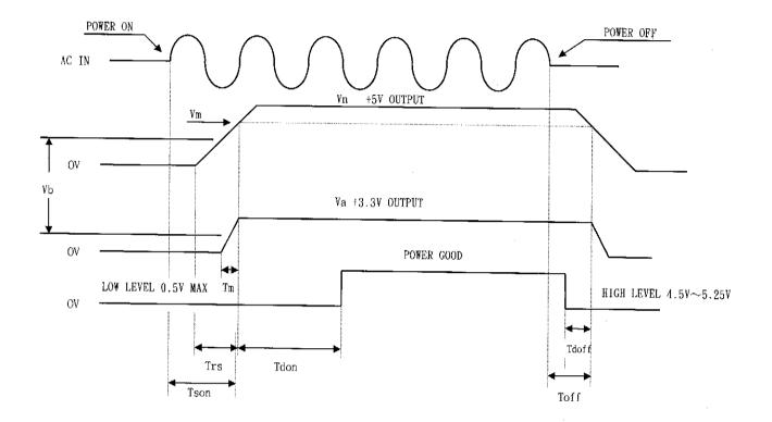
Vn Nominal voltages +5V Vm Minimum voltages +4.5V Va Nominal voltages +3.3V Vb +2.0V max Tson Switch on time (2000 ms. max.) Trs +5V rise time (50ms. max.) Tdon Delay turn-on (100ms. < Tdon < 500ms.) Tdoff Delay turn-off (1 ms. min.) Toff Hold up time (16ms Min)
