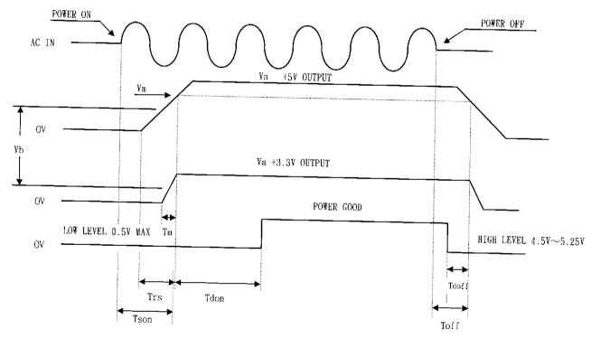
Vn Nominal voltages +5V Vm Minimum voltages +4.5V Va Nominal voltages +3.3V Vb +2.0V max Switch on time (2000 ms. max.) Tson +5V rise time (50ms. max.) Trs Delay turn-on (100ms.  $\leq$  Tdon  $\leq$  500ms.) Tdon Delay turn-off (1 ms. min.) Tdoff Toff Hold up time (16ms Min)
