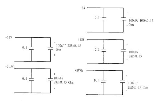
0.1uf is ceramic, the other is electrolytic capacitor. Noise bandwidth is from DC to 20Mhz
