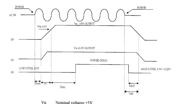
Vm Minimum voltages +4.5V Va Nominal voltages +3.3V Tson Switch on time(500ms. Max) Trs +5V rise time (100ms. max.) Delay turn-on (100ms. < Tdon < 500ms.) **Tdon** Tdoff Delay turn-off (1 ms. min.)
