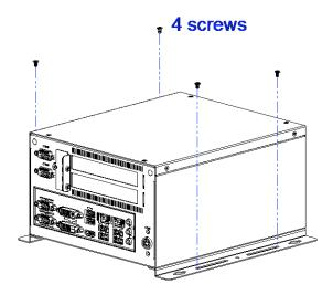
You can install CMI212 System on plastic (LCD monitor), wood, drywall surface over studs, or a solid concrete or metal plane directly. The types of fasteners required are dependent on the type of wall construction.
