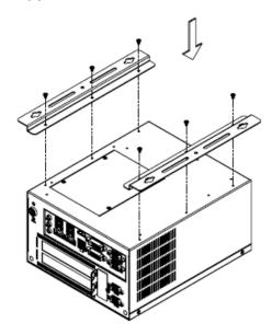
2. Prepare at least four screws (M3, 6 mm) to mount the device on wall .
