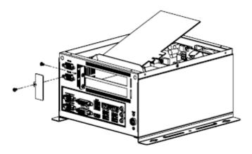
3. Fix the card by tightening the screws mentioned above.
